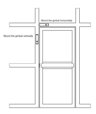
Center the gimbal mount to mounting surface and mark the mounting holes for the gimbal mount on the surface.
