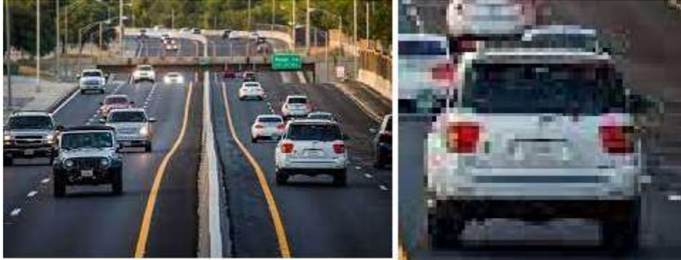
The zoom lens has the ability to get the best field of view since it can be adjusted to get a largest view of the plate. It is best to try for a minimum of 80 pixels per foot.
