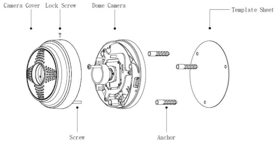
4. Assemble Camera Cover to Dome Camera. Turn the Camera Cover clockwise to complete installation.
