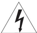
The lightning flash with arrowhead symbol, within an equilateral triangle, is intended to alert the user to the presence of dangerous voltage within the products enclosure that may be of sufficient magnitude to constitute a risk of electric shock to persons.
