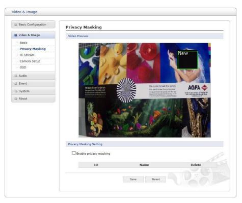
The privacy masking function allows you to mask parts of the video image to be transmitted. You can set up to eight privacy masks.
