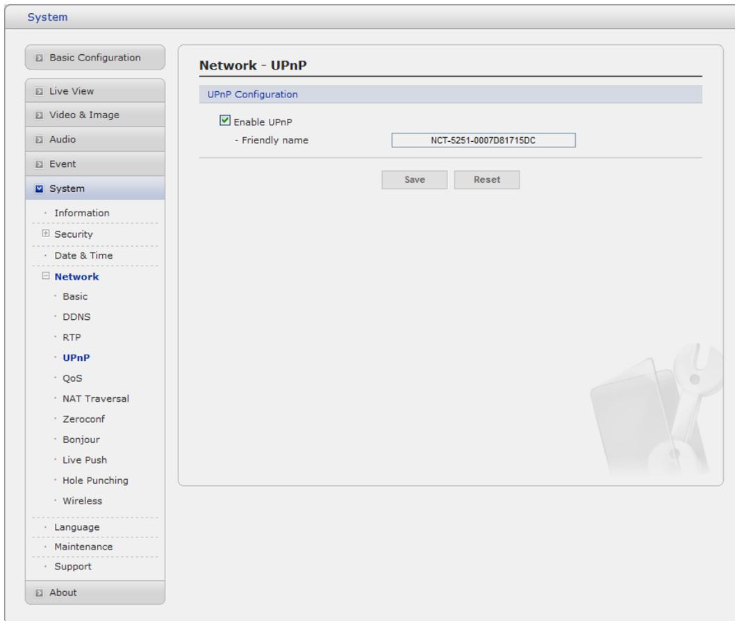
The Network Camera includes support for UPnP™. UPnP™ is enabled by default, and the Network Camera then is automatically detected by operating systems and clients that support this protocol.
