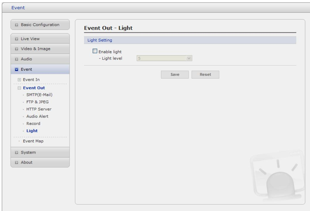
The LED on the front of the camera can be set to flash at a configurable interval when an event is triggered. From the Activate drop down menu, select a Light level which the LED will brighten to.
