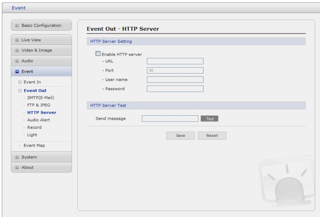
When the network camera detects an event, HTTP Server is used to receive uploaded image files and/or notification messages. Check the box to enable the service.
