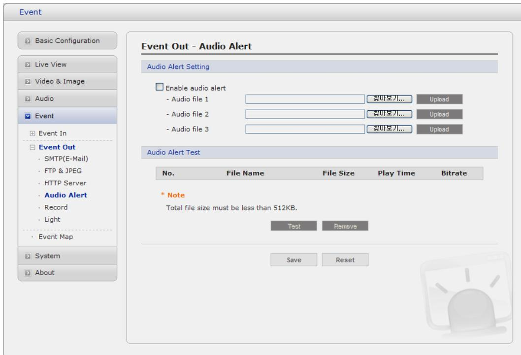
When the network camera detects an event, it can output a predefined audio data to external speaker. Check the box to enable the service.
