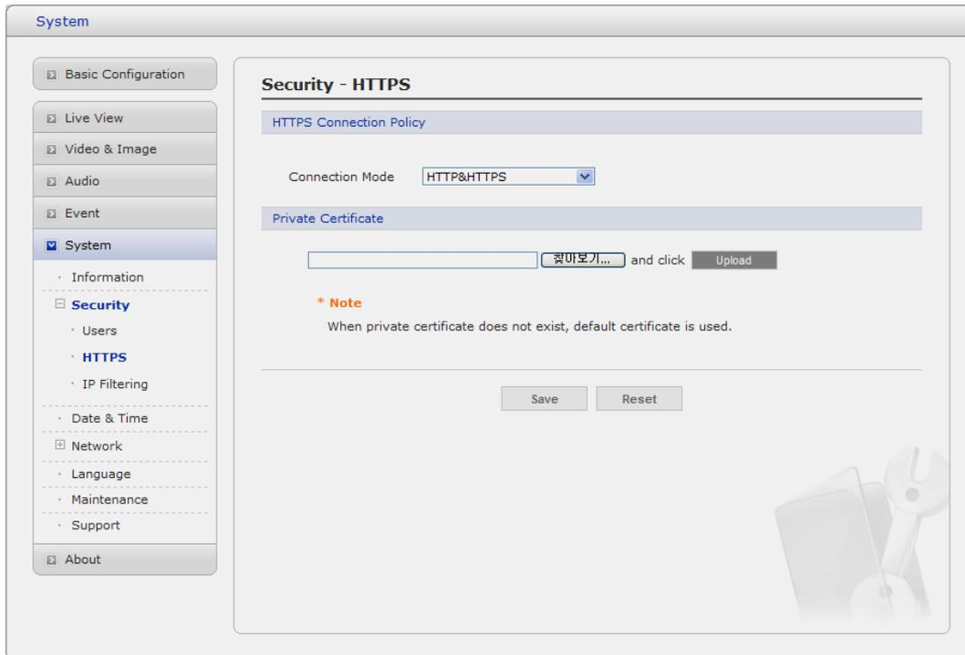
For greater security, the Network Camera can be configured to use HTTPS (Hypertext Transfer Protocol over SSL (Secure Socket Layer)). That is, all communication that would otherwise go via HTTP will instead go via an encrypted HTTPS connection.
