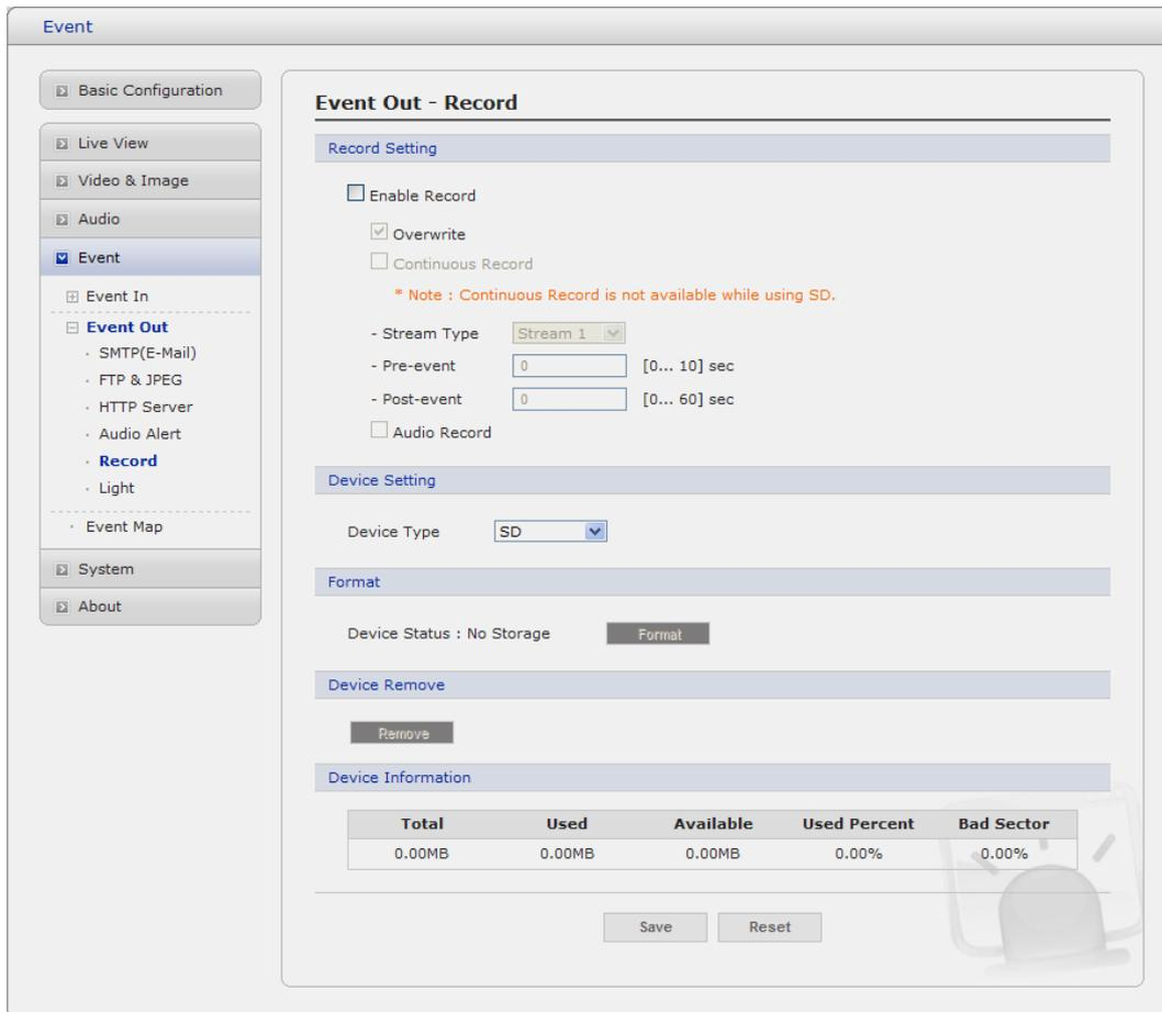
When the network camera detects an event, it can record video stream in the Micro SD Memory (not supplied) or NAS (Network Attached Device) as a storage device. Check the box to enable the service.
