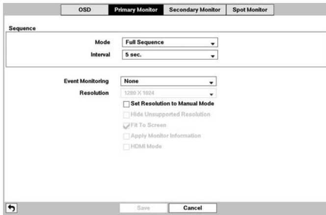
Figure 36 : Display – Primary Monitor setup screen.
