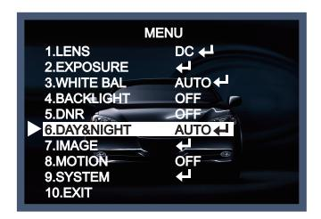
◆ AUTO : Automatically, It shifts into the color mode in the bright environment and the B/W mode in the low light condition. It can adjust the delay time, starting brightness and end brightness according to the ambient conditions by pressing the Set button.
