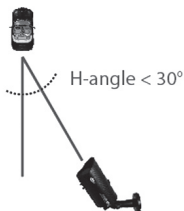
H-angle less than 30° correct
