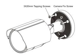
Camera Fix screws(2X) and align the bullet camera with it like above picture.
