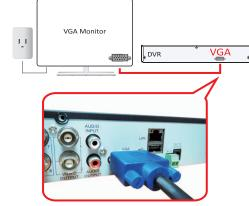
Plug a VGA cable from VGA monitor into the port marked "VGA" on the back of the DVR.
