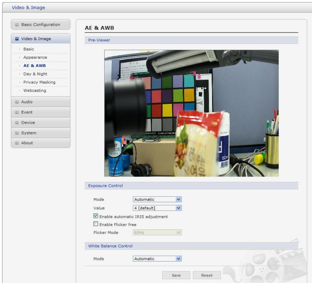
This page provides access to set the exposure and white balance of the network camera.
