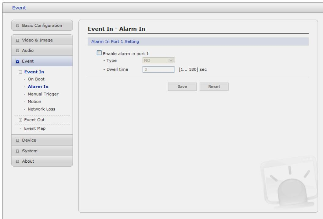
Select "Enable" to activate the alarm event. The network camera supports 1 alarm input port.
