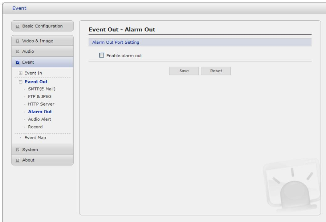
When the network camera detects an event, it can control external equipment connected to its alarm output port. Check the box to enable and then select either:
