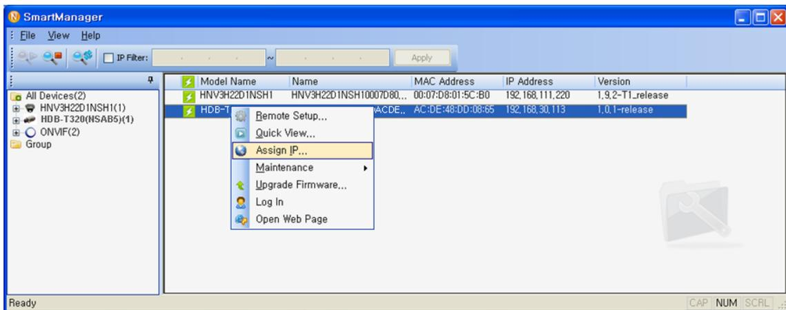
4. Select Assign IP. You can see a Assign IP window. Enter the required IP address.
