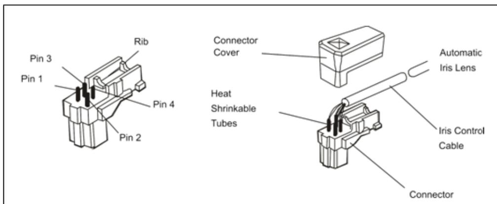
1. Solder the lens control wires to the connector supplied with the camera.
