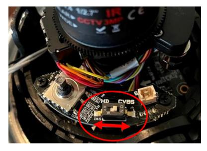
Camera Setup / Control on CVBS or when a recorder does not support control over COAX: When setting up a camera the internal joystick can be used to enter the menu to make setup changes or prior to entering the menu to make changes to zoom/focus if equipped with a varifocal lens.
